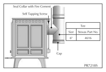
1.7 Connect a tee by inserting it into the flue spigot and sealing using fire cement and secure with a suitable self tapping screw. The cap supplied with the tee is used as the cleaning access. **Do not use a 90° elbow to make this connection**.
